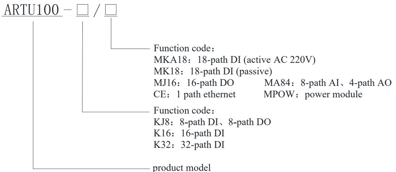
Note: MPOW power module must be selected when module is selected.
